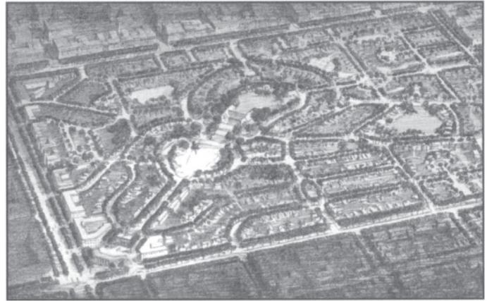
The neighborhood unit. 160 acre tract for 6000 people with pedestrian ways for dwellings, school, and shops with no transecting highways. Drawing: Chester B.Price, House and Garden , 1925
